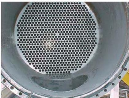
**Top photo: A heat exchanger tube sheet before water blast cleaning. Bottom photo: The same heat exchanger tube sheet after cleaning.**
